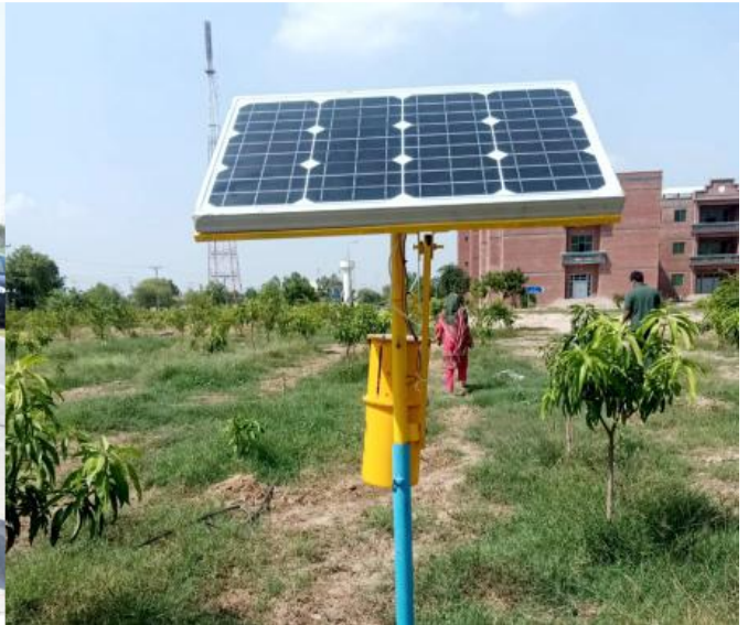
Solar based Smart trap for insect detection
